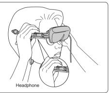
When you remove the display unit, some types of glasses may come off together with the display unit. To avoid this, move the bridge of the glasses in the direction of the arrow as shown.
